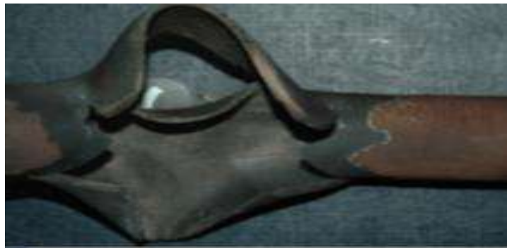
SH LT OVERHEATING (SHORT-TERM OVERHEATING)
